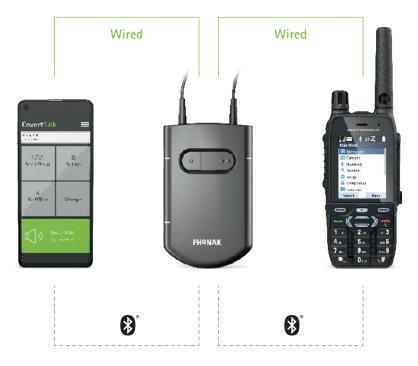
Roger<sup>™</sup> Covert C can handle one Bluetooth<sup>®</sup> link while Roger<sup>™</sup> Covert Dual C separable can simultaneously handle one Bluetooth<sup>®</sup> link and one separable wired link.
